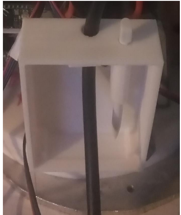
Figure 30: Display housing before the display is installed
